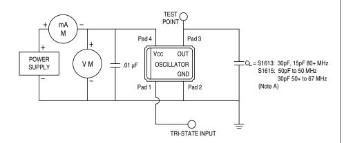
Note A: C<sub>L</sub> includes probe and jig capacitance.
